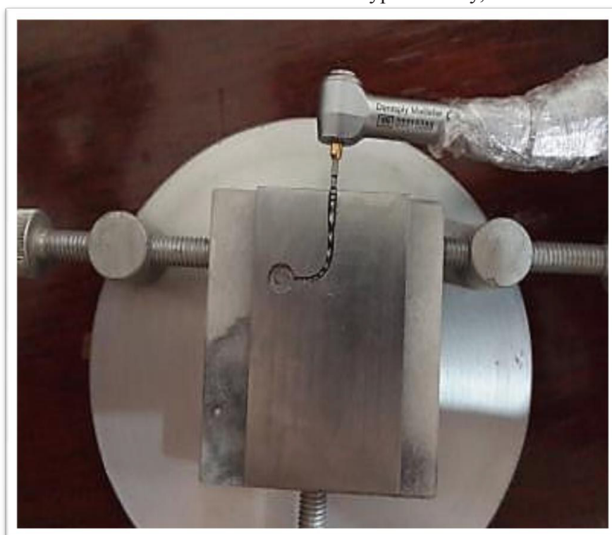
Figure 1. The static model used for cyclic fatigue testing.
